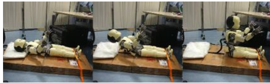
Fig. 14. The demonstration of the learned sit-up motion by an actual robot.
