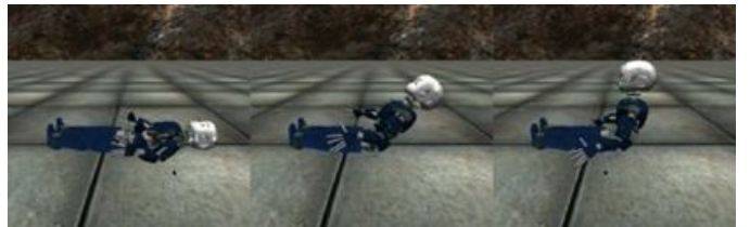
Fig. 4. The screenshots of the teaching experiment of the sit-up motion. The left figure shows the initial state. The figure in the center shows an intermediate state of lifting up. The right figure corresponds to the final state of the sit-up.
