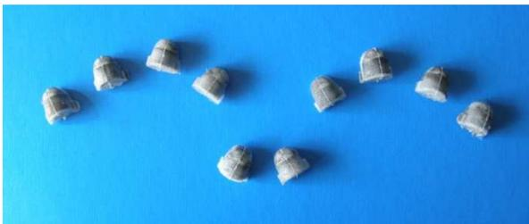
Figure 3 demounted fingertips used by the humanoid robot iCub during grasping tasks.
