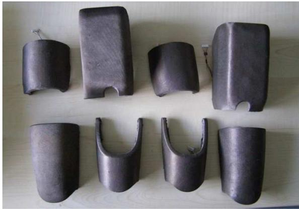
Figure 2 demounted cover of the upper arms and forearms implementing the artificial tactile skin of the humanoid robot iCub.
