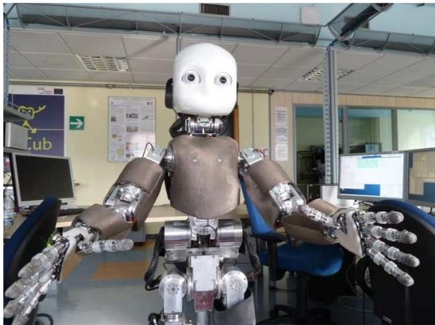
Figure 4 Humanoid robot iCub covered with artificial skin able to detect conductive and non-conductive materials (arms, torso, palms and fingertip)
