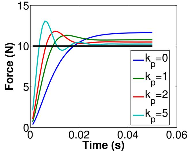
Fig. 3. Contact force with proportional feedback force control for different values of the proportional gain  $k_p$ .
