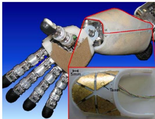
Fig. 2. Right arm of the iCub robot, with skin mounted on the forearm (not covered with the lycra yet), palm and fingertips. In the red box, a detailed view of the forearm cover and the placement of the sensors [15]. This part is not covered with the silicone foam yet.
