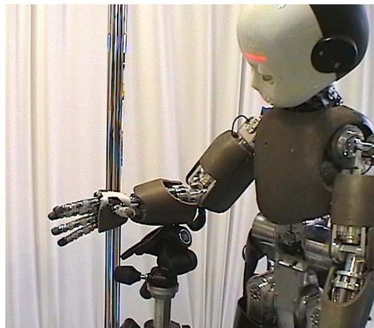
Fig. 1. The iCub robot, with skin mounted on the torso, arms, palms and fingertips. The iCub is sliding its forearm against the top of the tripod that is standing in front of it.
