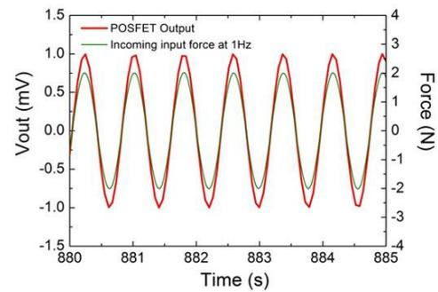
**Fig. 4. Flexible touch sensing device response for a sinusoidal signal of an amplitude of  $4\text{ N}$ , at a frequency of  $1\text{ Hz}$  measured with a  $V_{\text{ddl}}$  of  $13\text{ V}$  and an external load of  $2.7\text{ k}\Omega$ .**
