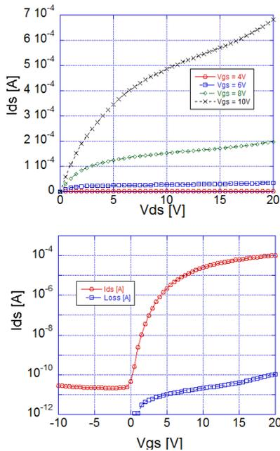
**Fig. 1. (a) Output characteristic for a TFT with  $W/L=40$ , (b) transfer characteristic of the same device, measured at room temperature after the detach from the rigid carrier.**
