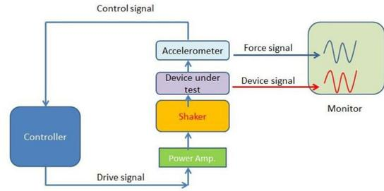
**Fig. 3. Schematic of the experimental set up used for the electromechanical test.**
