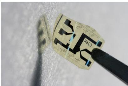
**Fig. 2. A photograph of the pressure sensor integrated with the LTPS TFTs fabricated on polyimide after the detach from the rigid carrier.**
