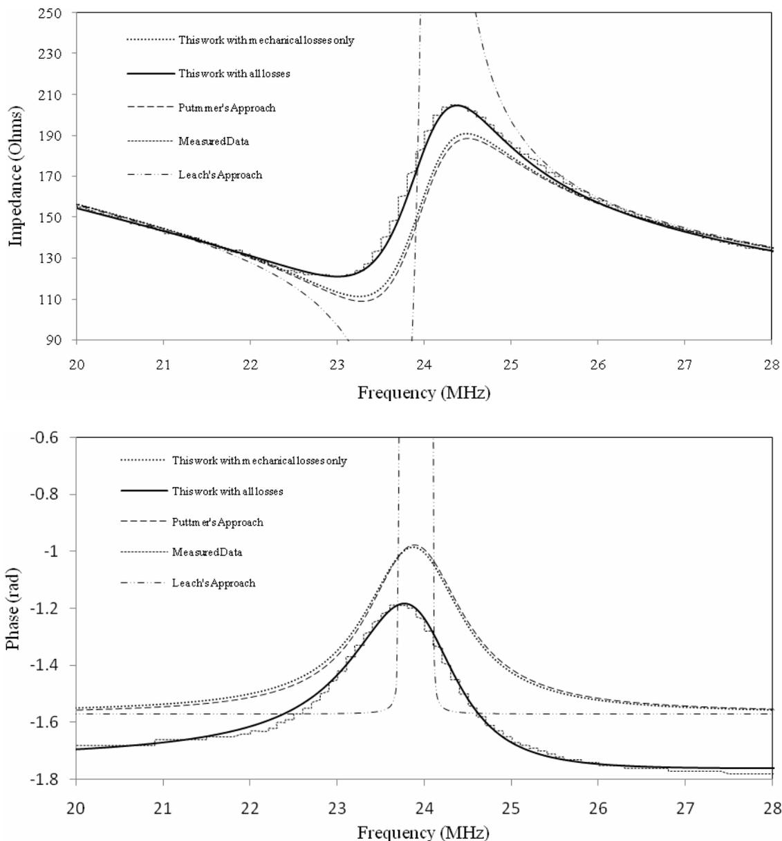
Fig. 3. Comparison of Impedance (top) and Phase (bottom) of the PVDF-TrFE sample.
