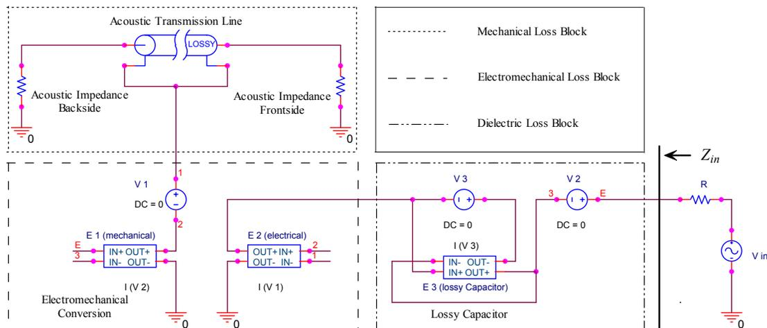
Fig. 2. Schematic of the equivalent model of piezoelectric polymer implemented with PSPICE. The model has been divided into various blocks showing the mechanical/acoustic/viscoelastic, electromechanical/piezoelectric and electric/dielectric losses.
