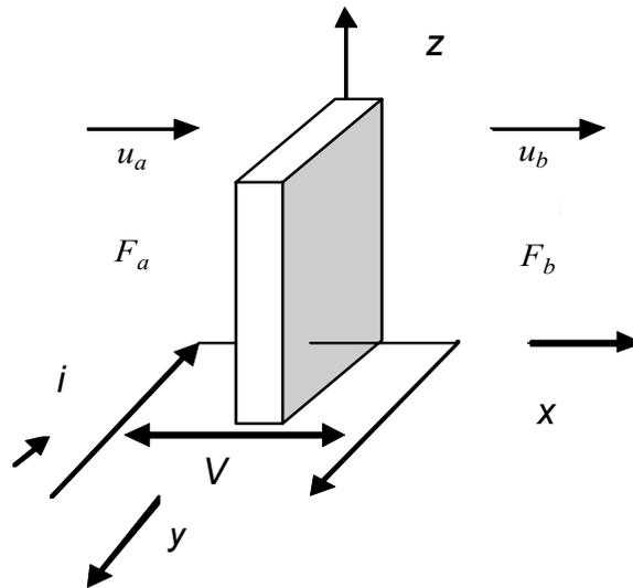
Fig 1. Piezoelectric polymer in thickness mode.
