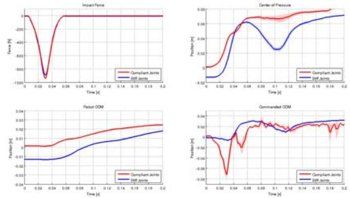
Fig. 10. The system response in the first 0.2 seconds after the impact (impact on the platform).
