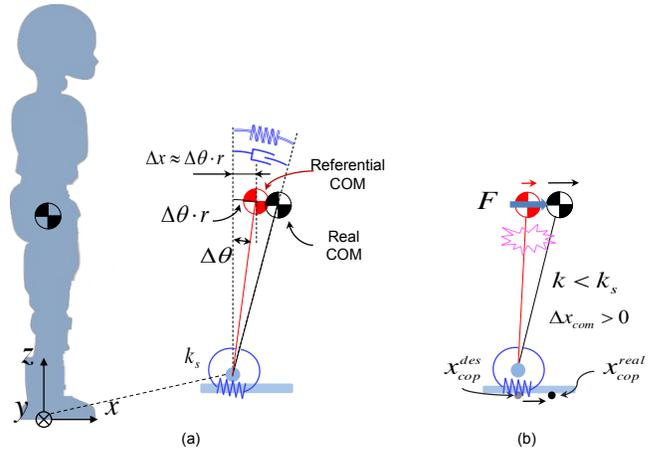
Fig. 4. Compliance control by regulating the COM reference
