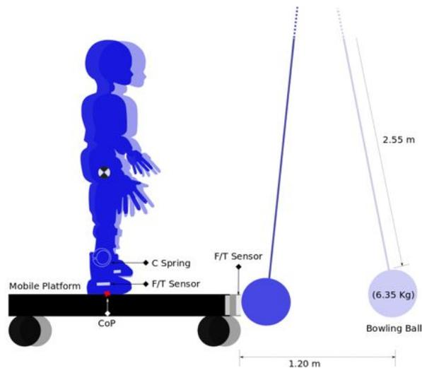
Fig. 9. A sketch of the second experimental scenario: impact on the platform.
