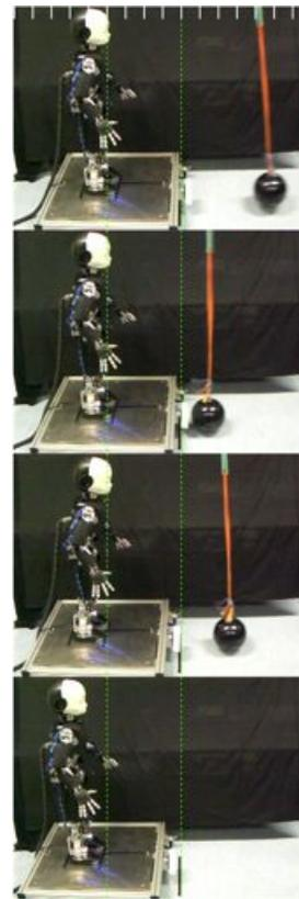
Fig. 11. A sequence of pictures showing the system balancing reaction after an impact on the support platform.
