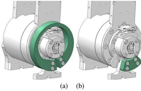
Fig. 3. Rigid joint substitution. The figure shows how by substituting the element connecting the motor output and the joint output it was possible to obtain a SEA joint (a) and a rigid joint (b) on the same setup.
