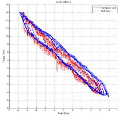
Fig. 5. The overall (active+passive) stiffness at the ankle joint. The gains of the balancing controller were experimentally tuned in order to achieve the same equivalent stiffness both with stiff and series elastic joints (stiff joint:  $K_p = 0.4$ ,  $K_d=0.005$ ; elastic joint:  $K_p=0.3$ ,  $K_d=0.08$ ).
