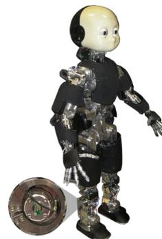
Fig. 1. A picture of the robot used in the experiments with a zoom on the series elastic element which was replaced with a rigid element during experiments with the rigid transmission.
