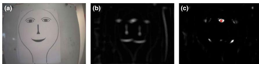
**Figure 3** Images taken from the robot during operation. (a) The Face stimulus. (b) Superimposed stereo pair. Note how the eyes overlap. (c) Result of pointwise multiplication of the stereo pair. Note how overlapping regions of activity in the stereo pair are amplified relative to the rest of the signal. The red circle indicates the point of maximum salience in the map.
