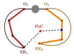
(a) Classical Approach: the two arms, with origins O<sub>1</sub> and O<sub>2</sub>, corresponding to the shoulders of the iCub, and end-effectors EE<sub>1</sub> and EE<sub>2</sub> located in the palms of its hands, are controlled in parallel.
