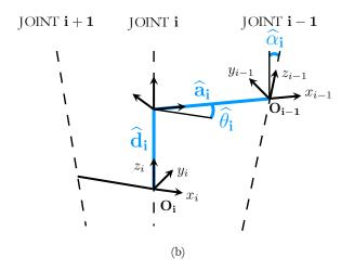
Fig. 4: Comparison between the original DH convention (a) and the proposed solution for the reversed chain (b). In order to "reverse" the original kinematic chain, the reference frames for the links have been kept coincident with the original ones.
