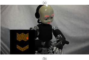
Fig. 2: **Self-touch experiment**. (a) The iCub touched on its left forearm by the experimenter; corresponding skin activation shown on the left. (b) The iCub touching the previously stimulated point using the index finger of the contralateral arm.
