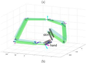
Fig. 5: **Optimization of the kinematic chain**. The chain is closed on one end through the skin (a fixed transformation from the taxel to the wrist) and through the index finger on the other end (another fixed transformation from the contralateral hand to the fingertip). (a) Schematic illustration of the framework. (b) Initial vs. optimized kinematic chain. The initial parameters (CAD values) shown in blue, the optimized in green.
