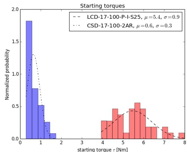
**Fig.4:** Starting torque test results. The figure shows the results of the starting torque test for the two actuators being compared. The corresponding normalized gaussians have been superimposed in the plot. Their corresponding averages and standard deviations are indicated in the legend.
