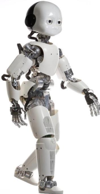
*Fig. 1: The iCub Humanoid robot*
