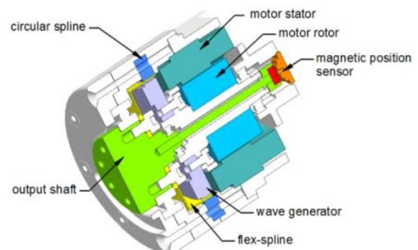
*Fig. 2: Cross section of the actuator under test*
