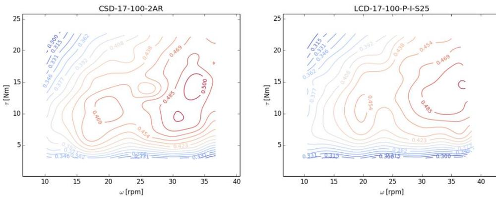
**Fig.6:** Actuators efficiency plots. The figure represents the contour plots of the averaged efficiencies as a function of the braking torque and the angular velocity.
