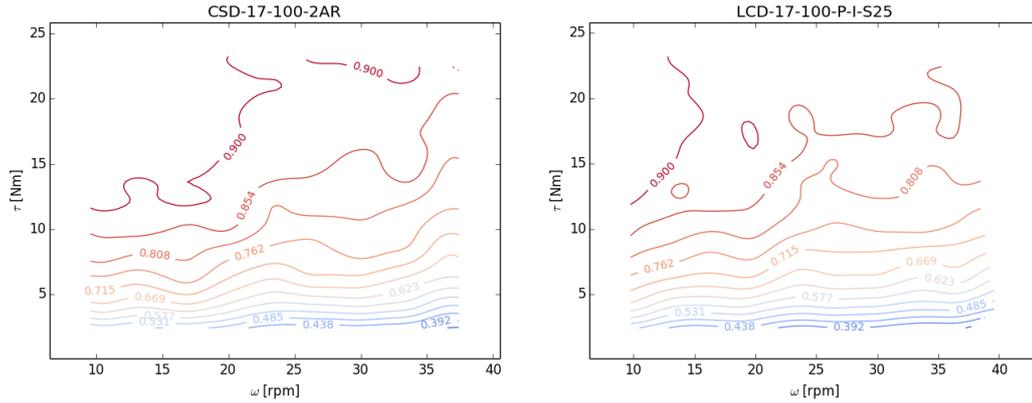
**Fig.5:** Transmission efficiency plots. The figure represents the contour plots of the averaged efficiencies as a function of the braking torque and the angular velocity.
