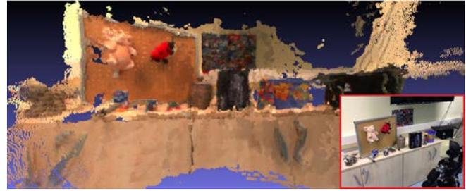
Fig. 10. 3D scene reconstruction obtained by moving the iCub head.
