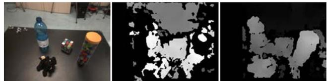
Fig. 2. Left: A typical scene as seen by the robot point of view. Middle: The depth map retrieved by the vision system based on pure kinematics calibration (producing poor results). Right: The improved depth map obtained after the calibration described in Section III-A.
