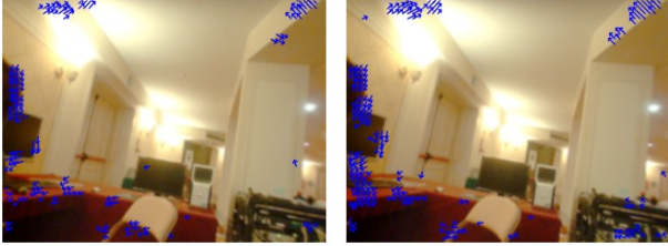
Fig. 4. Optical flow computed from two subsequent image frames from the left camera, iFB experiment (compensation using inertial feedback). Blue 2D arrows represent the optical flow vector \text{of}^t(u, v) at each pixel. For clarity optical flow vectors are reported only for a subset of the pixels (one pixel every five).
