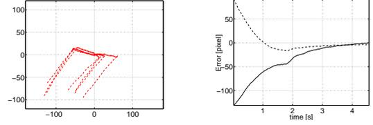
Fig. 5. Left: movement of the hand on the left image plane ( $320 \times 240$ ) during the execution of different reaching actions. Solid line: closed loop. Dashed trace: open loop. Right: time response of the closed loop and open loop strategy on the left image plane. Solid line:  $u_l$ . Dashed lines:  $v_l$ .
