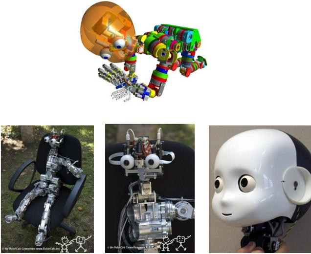
Fig. 1. Details of the *iCub* design and construction.
