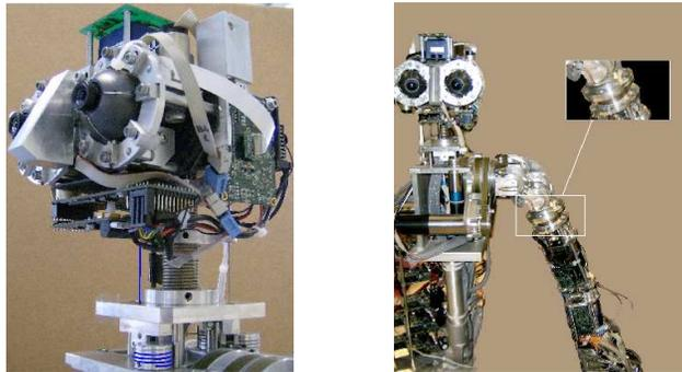
**Fig. 1.4.** Pictures of the vision (left) and force (right) sensors mounted on James. Vision is achieved with a stereo pair of digital cameras. External forces are instead measured with a six degrees of freedom force sensor placed in the forearm of the robot.
