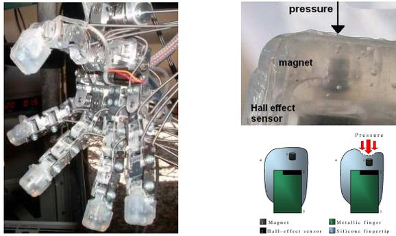
**Fig. 1.5.** Picture (left) and schematics (right) of the touch sensors mounted on the hand of James. Each fingertip has a couple of sensors based on a Hall effect technology. Eight more touch sensors are mounted on the phalanges.
