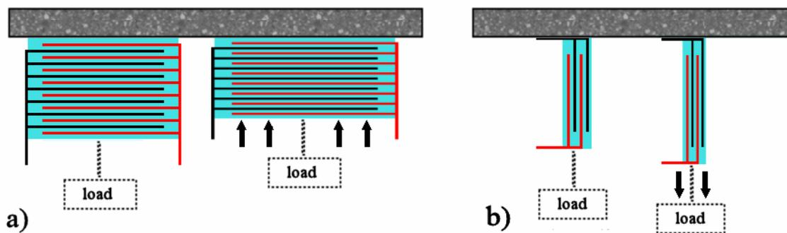
Fig. 2. Operation principle for multilayer DEAs used to produce contractile motion (a) and expanding motion (b).
