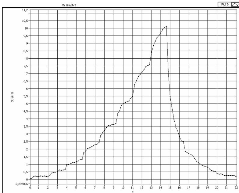
Fig. 11. Viscous behavior of an acrylic (VHB) DEA. Lateral strain is here presented vs time, in response of voltage steps of increasing magnitude.
