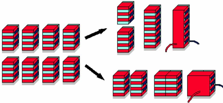
Fig. 8. Assembly of many independent contractile units in bigger actuators packaged in series or in parallel.
