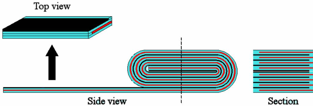
Fig. 3. A multilayer stack configuration obtained rolling the electroded dielectric film on a flat removable core.
