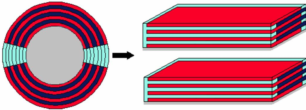
Fig. 9. Schematic fabrication of two expanding actuators (multilayer stacks) starting from the previously fabricated roll.
