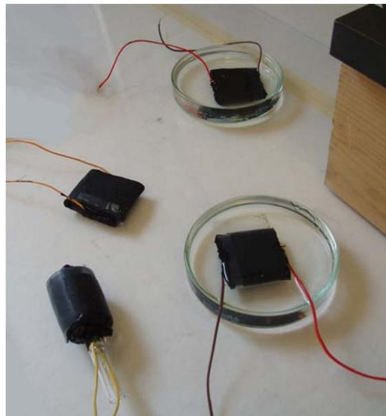
Fig. 4. Prototypal DEAs fabricated in different shapes and sizes.
