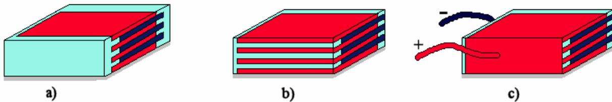
Fig. 6. Connection of the electrode layers. The inside structure of the stack is here exposed only for picture clarity.
