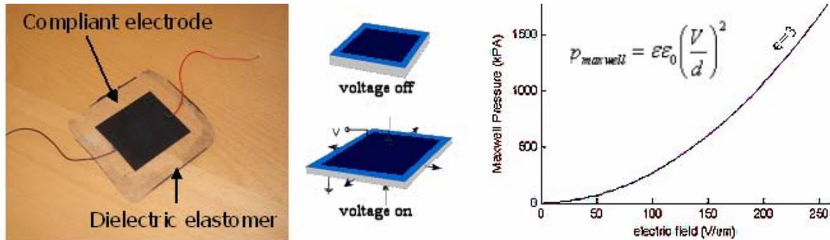
Fig. 1. Operation principle for a single-layered dielectric elastomer actuator and theoretical evaluation of Maxwell pressure in function of the applied electric field.
