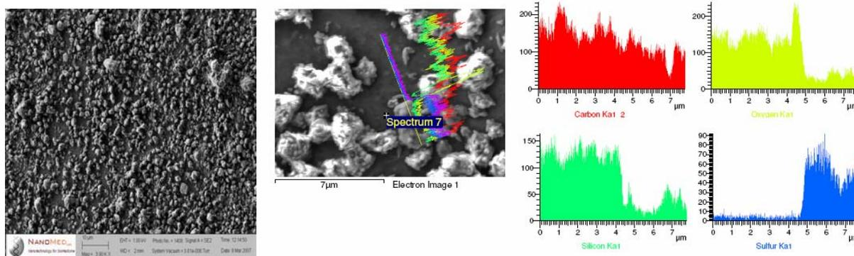
Fig. 12. SEM and X-Ray Microanalysis of the airbrushed compliant electrodes.
