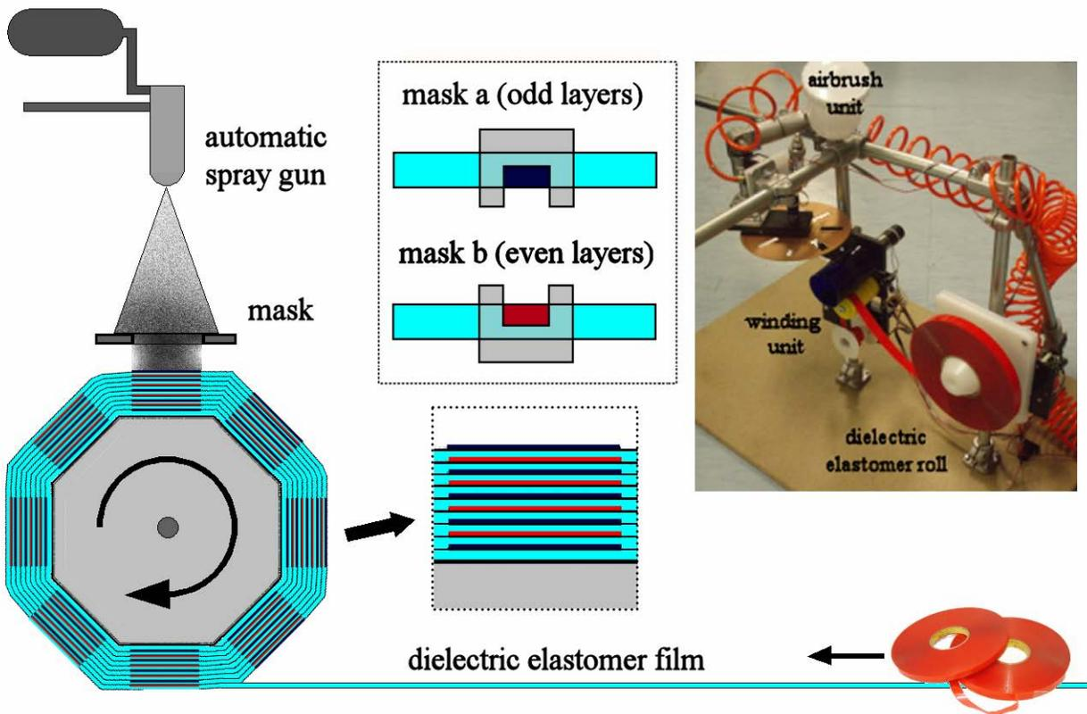
Fig. 5. Semiautomatic fabrication process of multilayer stack actuators.
