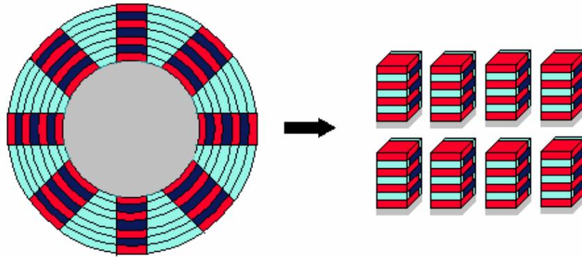
Fig. 7. Schematic fabrication of eight contractile actuators (multilayer stacks) starting from the previously fabricated roll.
