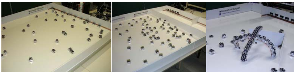
Figure 8: (a) Docking of a few robots for recharging. Shown is the two-line approach: the first line - recharging robots, the second line - robots waiting for recharging; (b) The "barrier problem" – robots separated from docking stations by a barrier; (c) Possible solution to the "barrier problem": swarm robots form a symbiotic multi-robot organism & collective pass the barrier.
