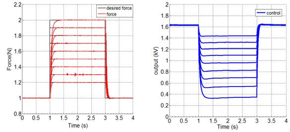
**Fig. 6:** Step response of the inner force control loop.
