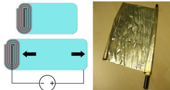
**Fig. 2:** Left: operating principle of an elastomer elongating roll actuator. Right: picture of the dielectric film employed in the device fabrication.
