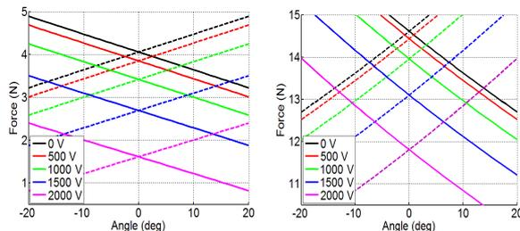
**Fig. 9:** Force-displacement planes for different levels of actuator preloads. The points where the lines intersect correspond to the equilibrium points of the joint. The angle between the actuators characteristics implicitly defines the joint stiffness.
