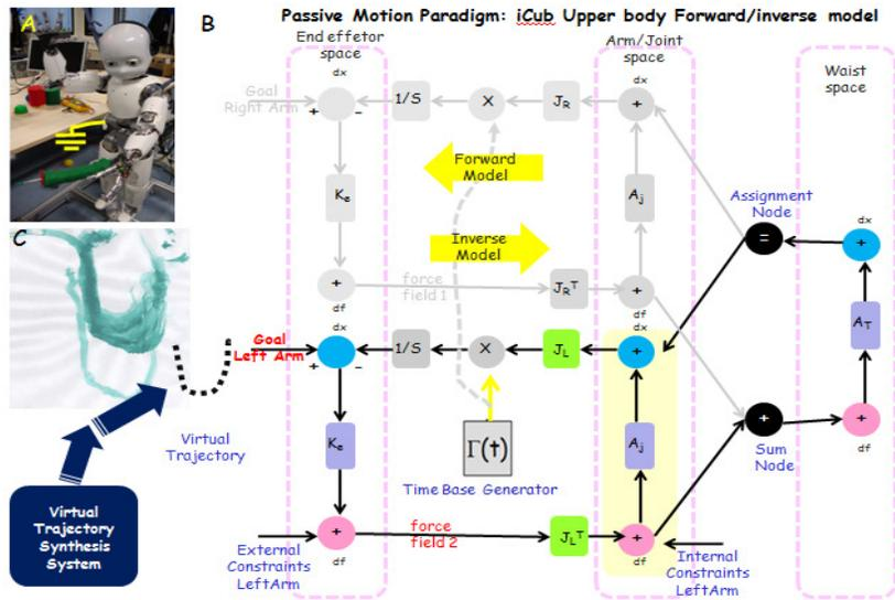
Figure 6. The PMP Forward/Inverse model for iCub upper body coordination. The torso/left arm chain is used in the iCub drawing experiments (Panel A), hence the right arm chain is deactivated. The evolving virtual trajectory acts as an attractor to the PMP system and triggers the synthesis of motor commands (This process is analogous to the coordinating a puppet, the VT serving the role of the puppeteer). Panel C shows the scanned image of drawings of iCub while learning to draw a 'U'.
