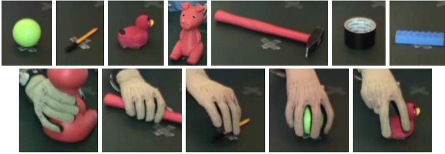
Fig. 3. Top row: the objects used in our experiments. Bottom, the grasp types we consider: (left to right) cylindrical power grasp, flat grasp, pinch grip, spherical and tripod grip.
