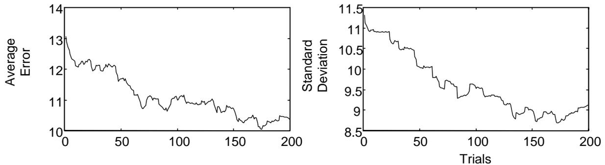
Figure 6: Robot motor performance. **Left:** moving window average of the residual retinal error (i.e. at the end of a fast motion). **Right:** the standard deviation of the same 300 samples. Abscissas represent the number of trials.
