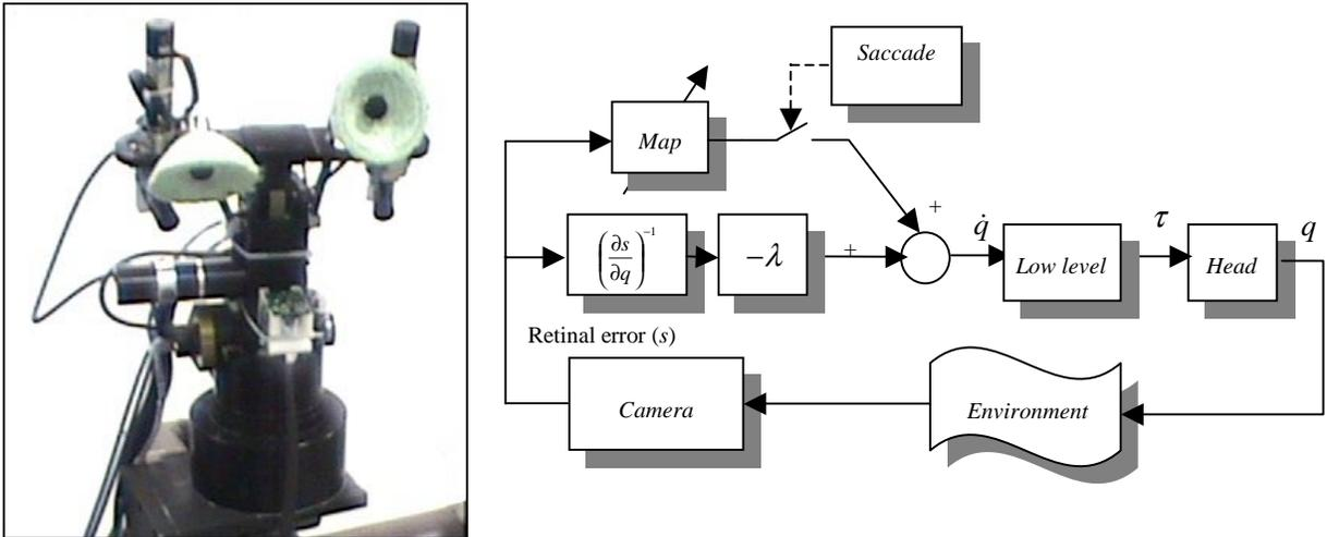
Figure 4. **Left:** the experimental set-up. **Right:** the robot control schema. It consists of a closed loop and a feed-forward secondary loop. The block identified by “Map” represents the GNG-Soft network.
