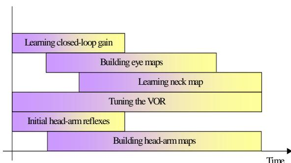
Figure 2 The developmental stages. The diagram above roughly shows the interleaving of the developmental stages; abscissa represents time. The first step is the acquisition of the closed loop gains; reflex-like modules control the arm sub-system. After a while, learning of the saccade control begins. Eventually the eye-head coordination is acquired together with a more effective head-arm coordination map.
