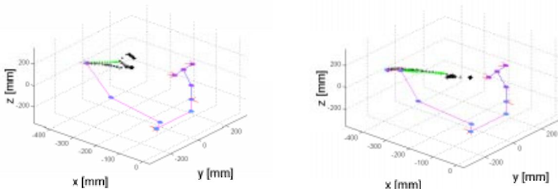
Figure 9 Reaching trajectories: two representative trajectories of the robot behavior. Two different marks can be distinguished: the crosses mark smooth pursuit control; the small squares are related to saccadic control. Note as in the leftmost picture the end-point and fixation position almost coincide.
