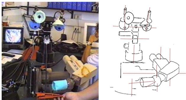
Figure 1 The experimental setup. Dashed lines on the rightmost picture represent the axes of rotation.
