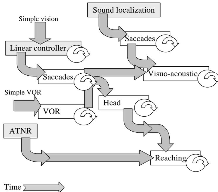
Figure 2 The developmental progression of the Babybot. A representation of how the various phases of the robot's development are interrelated. The light gray blocks are the initial configuration. See text for description of the learning blocks.
