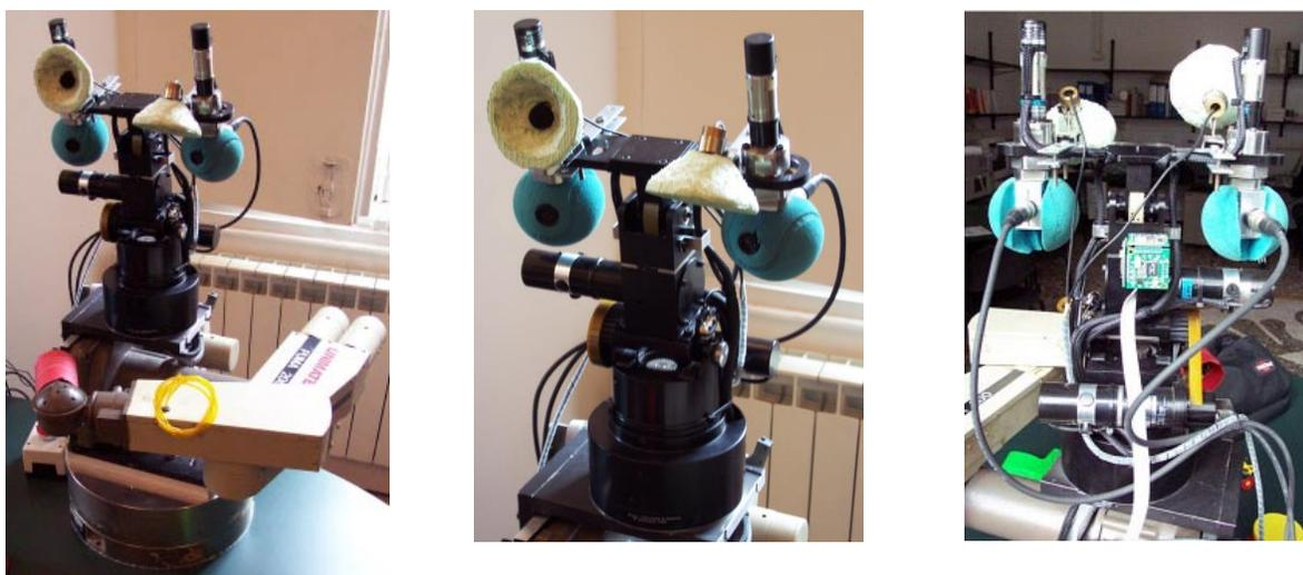
Figure 1: Three shots of the experimental setup. *Left*: complete view of the robot; *middle*: close up view of the head, note the cameras and microphones with earlobes; *right*: rear view of the robot and in particular of the gyros.
