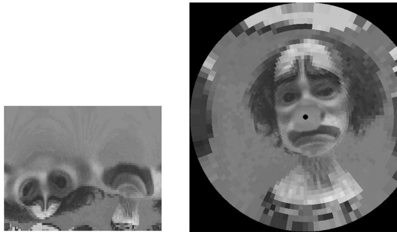
Fig. 2. The space-variant image geometry. *Left*: log-polar image of  $128 \times 64$  pixels. *Right*: the corresponding reconstructed Cartesian image.
