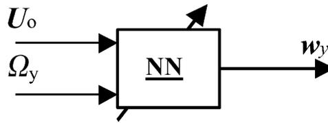
Fig. 2. Block diagram of the network inputs and output. The motion related sensory signals, the residual optic flow  $u_0$  and the head's angular velocity  $\Omega_y$ , are combined to produce a motor command, the compensatory eye movement  $w_y$ .
