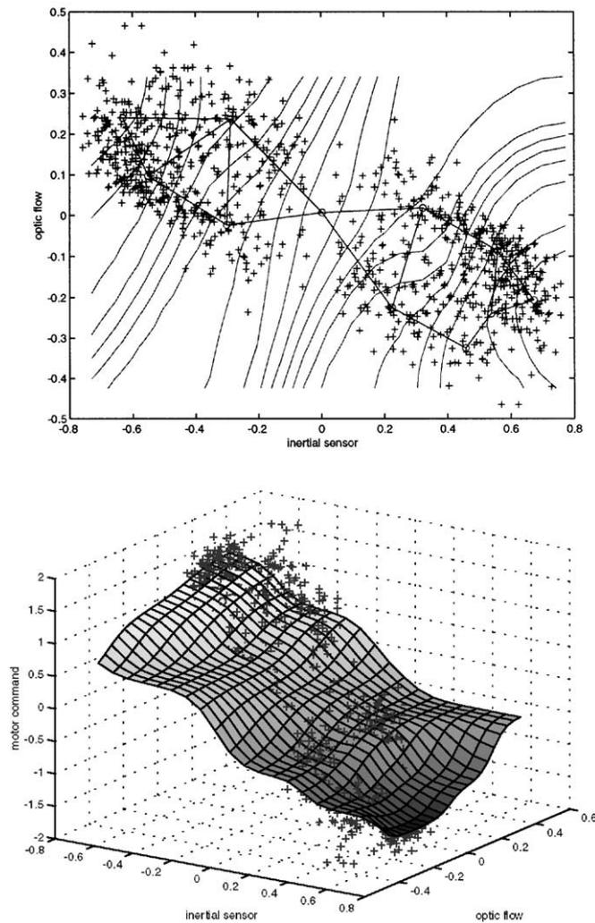
Fig. 4. The sensori-motor map of the stabilization reflex. Top: the distribution of the network units (light gray circles) in the input domain ( $x$ -axis inertial,  $y$ -axis optic flow). Bottom: the control surface representing the compensatory motor command ( $w_y$ ).
