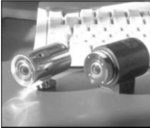
**Fig. 8.** Two different prototypes of the latest version of the Giotto camera. Both cameras are shown with a wide field of view lens ( $140^\circ$ ). The rightmost model has a standard C-Mount for the lens
