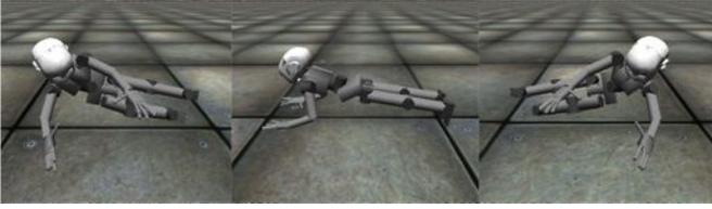
Fig. 3. Base motions. Right, front, left base motion from left to right.
